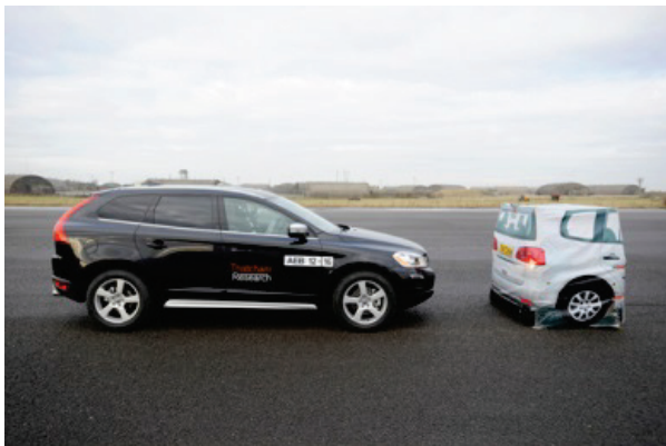
Figure 1: Volvo XC60 AEB test at Thatcham Research
